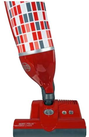
**Full Bag or Clog Indicator** – When a full bag, a clog in the airflow pathway, or an excessively dirty microfilter is detected, an indicator window on the bag housing lid fills with orange color and an airflow bypass valve opens, to prevent overheating and motor damage from a lack of adequate airflow.
