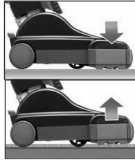
**Brush Adjustment Indicator Lights –** Two green lights, one for “up” and one for “down,” illuminate to indicate when the power head is adjusting the brush height to the proper cleaning level. Optimal cleaning effectiveness occurs when both lights are off.
